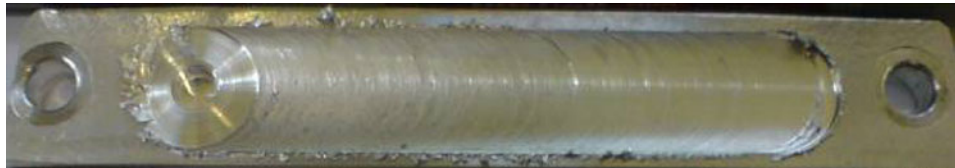
Fig. 2 Top face of the specimen produced by FSP
